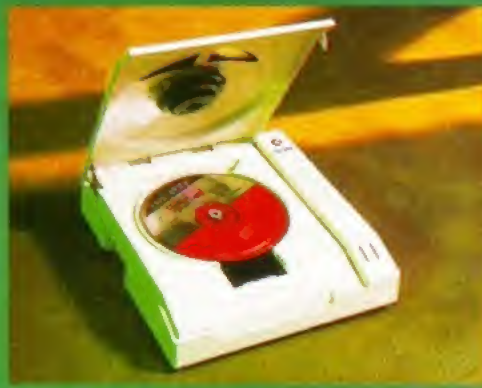
The A1200 CD-ROM drive has faster transfer rates than a CD 32 connected to an A1200 with ParNet.
